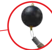
Floating Intake The ball float allows the pump to draw in clean water via the sieve which sits around 300mm below the top water level under the float.
